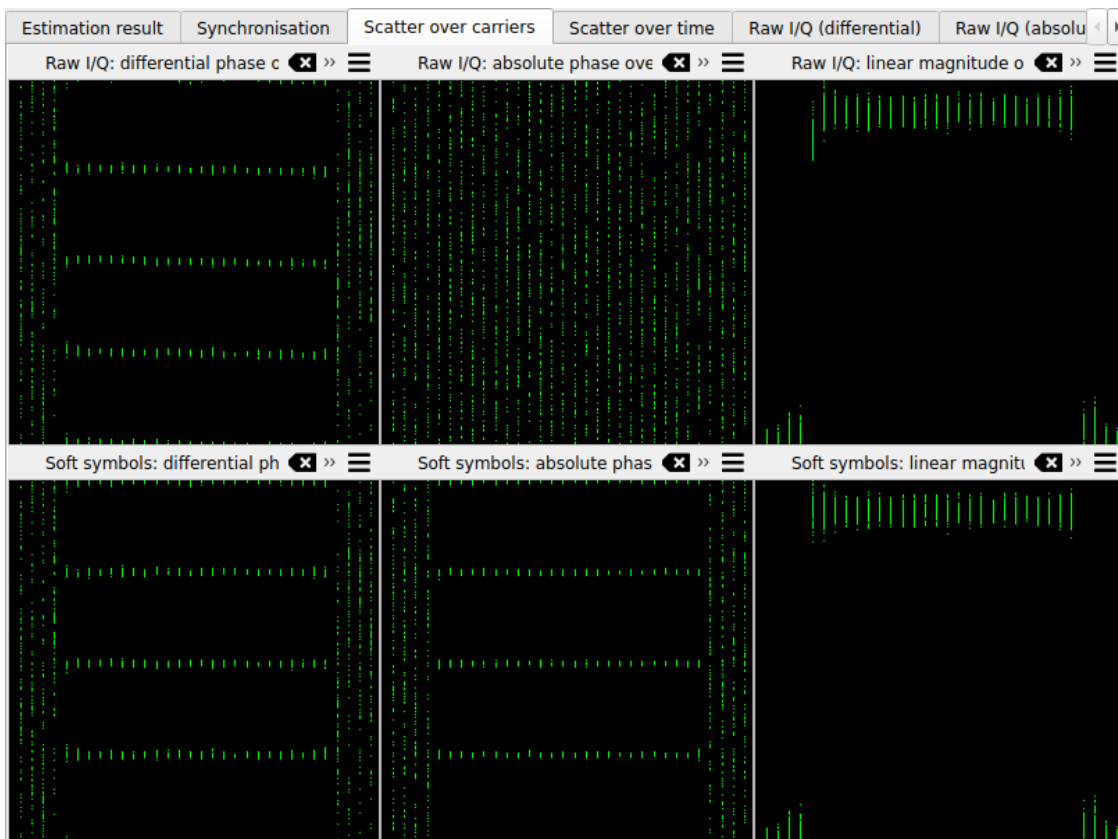
Figure 46: Example output of scatter diagrams over carrier number (i.e. frequency)
