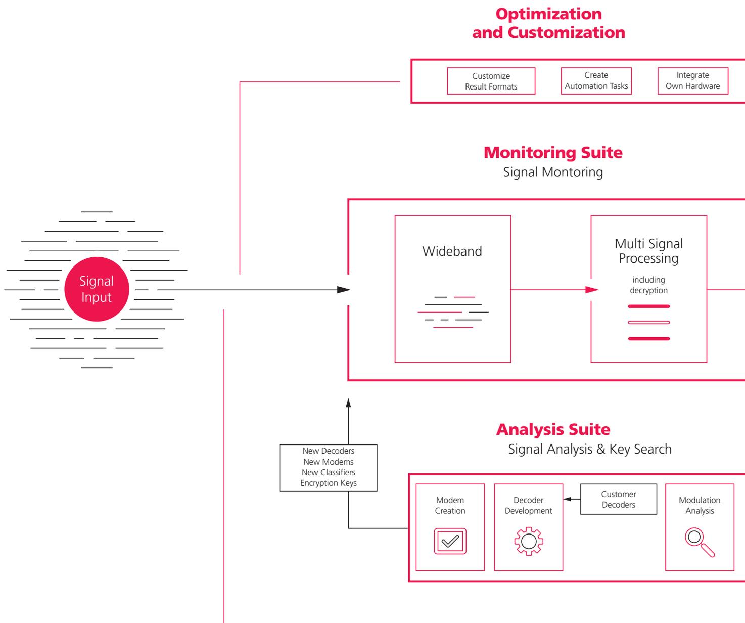
The Analysis Suite helps to adapt to new and unknown signals by creating new classifiers and decoders. With the ability to import them into the Monitoring Suite workflow to improve its capabilities.
