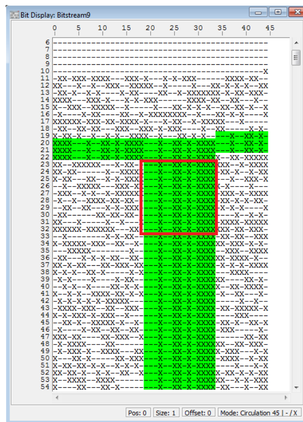
Figure 220: HFDL-Signal with periodic training sequences
