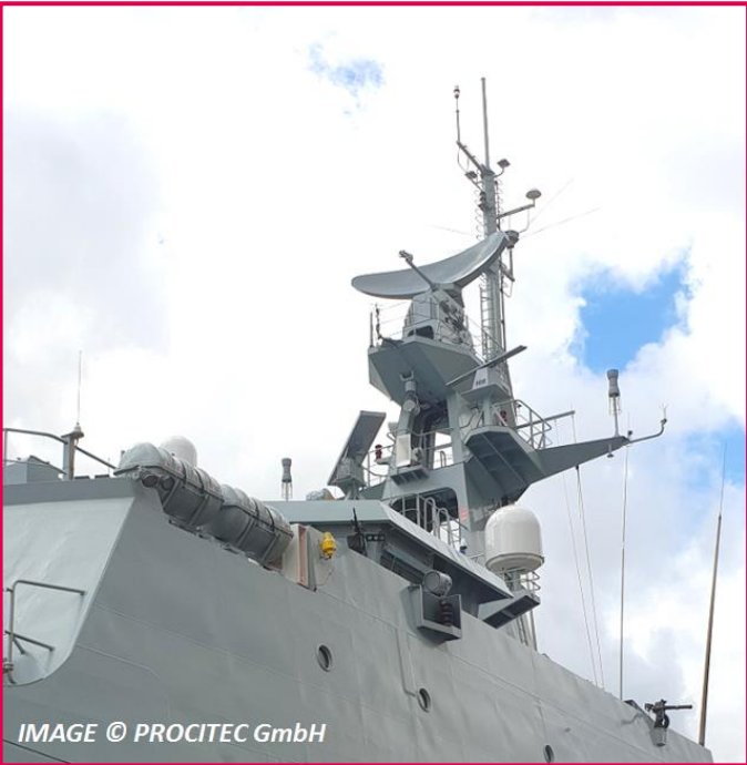
Mainmast with antennas on Offshore Patrol Vessel (OPV displacement 2000 Tonnes / Length 90 Meters [range 5500 nm] in this example)
