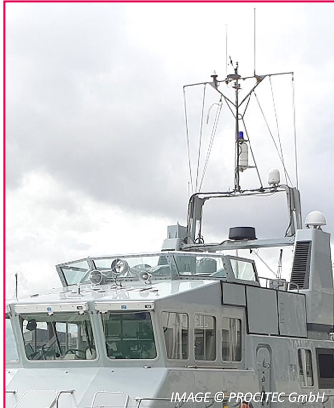
OPV mainmast showing V/UHF communications & intercept antennas (OPV displacement 54 Tonnes / Length 20 Meters [range 300nm] in this example)
