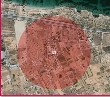
The image (left) illustrates coverage approximation for a range of 550 m at a sub-tropical land/littoral Area-Of-Interest (AOI) using the field-trial's low-cost/low-SWaP Wideband Receiver and roof-mounted UHF whip-antenna.
