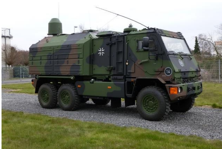
Figure 4: The system MoGeFA was introduced into the Bundeswehr for tactical V/UHF frequency spectrum monitoring and direction-finding
